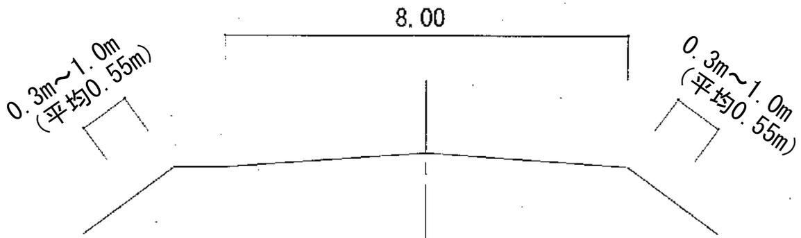
$$A = (1,350^{\text{上}} + 1,350^{\text{下}}) \times 0.55 \times 2^{\text{回}} = 2,970\text{m}^2$$
