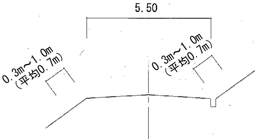
$$A = (1,600^{\text{上}} + 1,600^{\text{下}}) \times 0.7 \times 2^{\text{回}} = 4,480\text{m}^2$$
